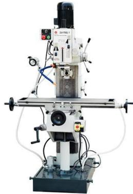
**Figura 14.1** Taladro Fresador
